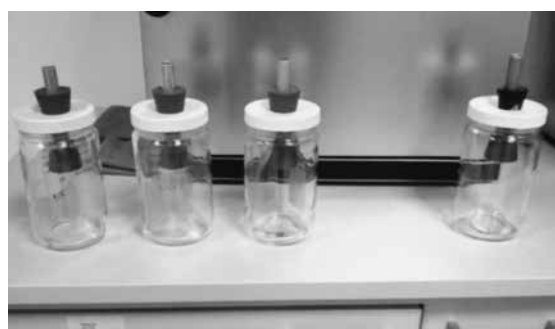
Figure 9 Plugs in glass jars with inhibitor
