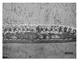
Figure 5 Laser spot diameter
