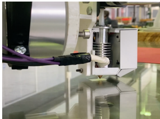
Figure 39: UR10e printing the first layer of the infill of a cube
