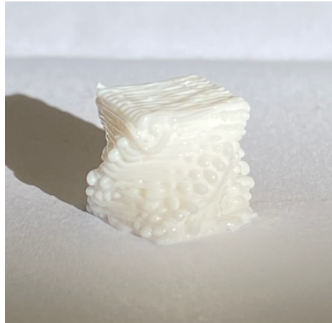
Figure 46: Printed 90° spiral cube with optimal speed parameters
