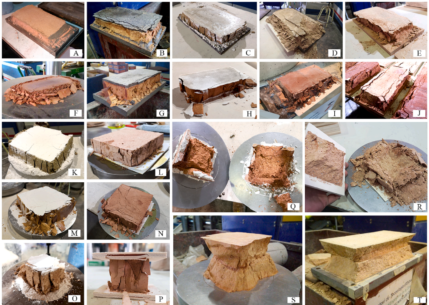
Fig. 4. Observed failure modes in the specimens with all bearing surface types. Handmade bricks ‘Mo’ from (A) to (E), (K), (L), (O), (Q), and (R). Mechanically extruded bricks ‘Ex’ from (F) to (J), (M), (N), (P), (S), and (T). (A) and (F) grinded, (B) and (G) capped with cement mortar, (C) and (H) capped with gypsum plaster, (D) and (I) placed with sheets of plywood, (E) and (J) placed with sheets of fibreboard, (K) and (M) covered with gypsum powder, (L) and (N) placed with two oiled PTFE leaves. (O) ‘Mo’ ‘C40’ covered with gypsum powder, (P) ‘Ex’ ‘C40’ placed with sheets of plywood, (Q) ‘Mo’ ‘100’ capped with gypsum plaster, (R) ‘Mo’ ‘100’ placed with plywood sheets, (S) Ex ‘2ha’ grinded and stacked. (T) Mo ‘2wh’ grinded and stacked.
