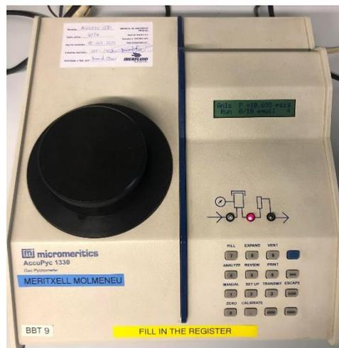
Figura 34: Accupyc 1330 Helium Pycnometer, Norcross, GA, USA
