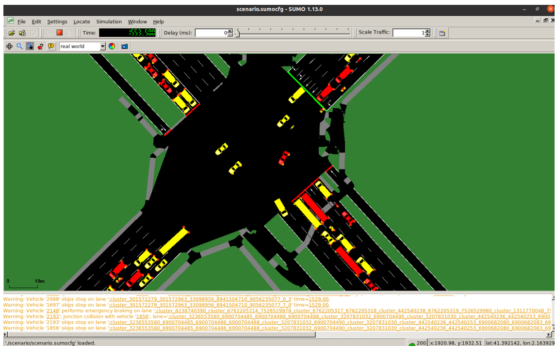
Figure 17: SUMO simulation of the collision scenario.
