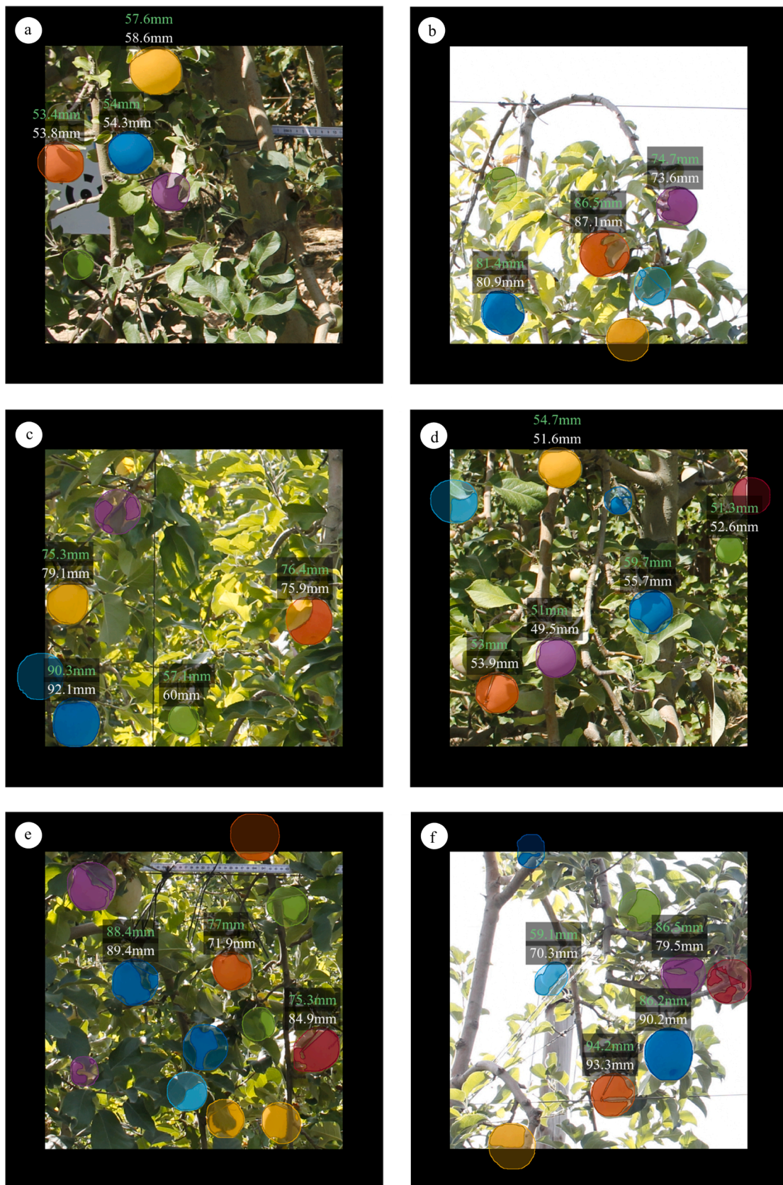
Fig. 12. Fruit detection and sizing results. Predicted diameters are provided for detections with an estimated visibility higher than 60%. Fruit size predictions are written in white and the ground truth in green. First row (a, b) contains examples of the best size estimation result, the second row (c, d) shows two intermediate scoring images and the third row (e, f) shows the two images with the worst estimations. (For interpretation of the references to colour in this figure legend, the reader is referred to the web version of this article.)
