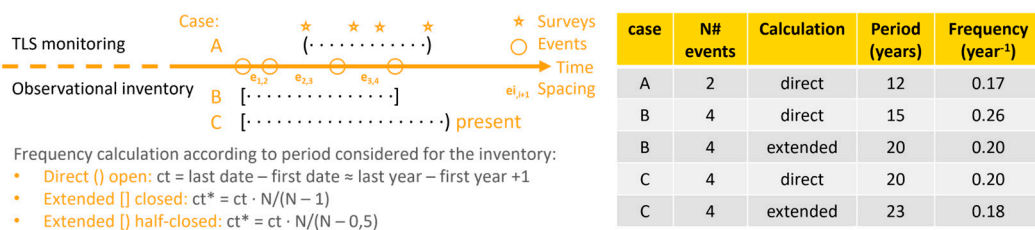
Figure 9. An illustrative example of the frequency calculation considering the covered period is as follows: In the case of A, the period of TLS monitoring is derived from the surveys and is not influenced by the occurrence of events, and its frequency can be directly calculated from ct ; in the case of B, if we consider the period fitted by the first and last recorded event, the frequency is over-estimated and the period must be extended to ct^* ; similarly, in the case of C, if we consider the period between the first record in the past and present time, the period should be extended by half due to an extreme fit by sampled data.
