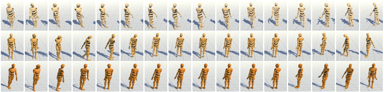
Figure 6: Three avatars animated with the same input (user doing a turn-in-place), but using an increasingly large portion of the animation database. From top to bottom: 10%, 25% and 100% of the poses in the database. Smaller databases struggle to match the user's motion, thus reducing the final quality and increasing the time and space needed to complete the turn.
