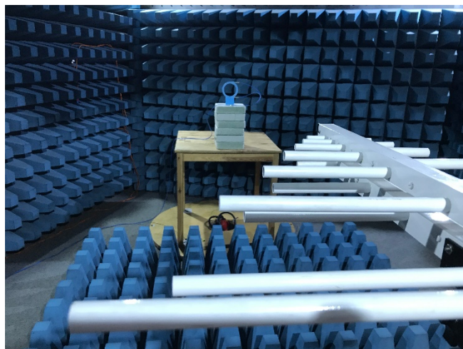
Fig. 5. Test set up in the anechoic chamber.
