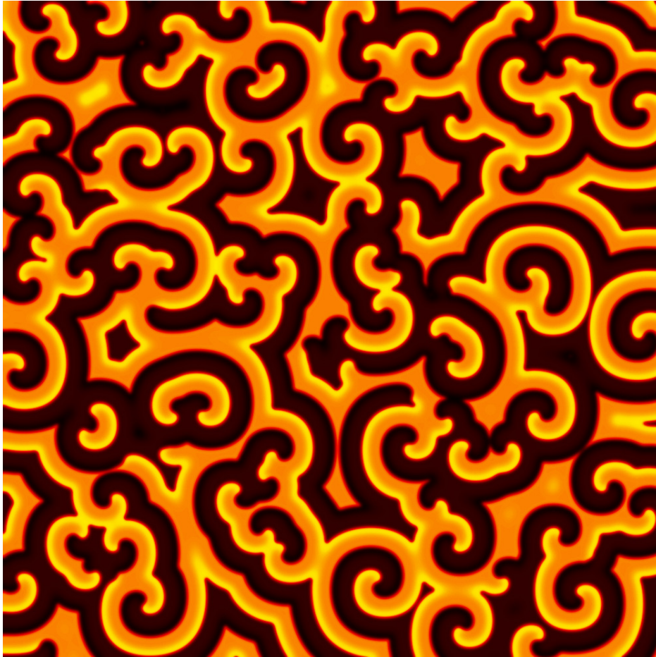
Fig. 2. Multiple spiral waves formation under random initial conditions in an excitable model. Several spiral waves rotate simultaneously with the same frequency in an homogeneous extended system generated by a set of random initial conditions. Waves are obtained in a model of chemical waves in microemulsions, however, similar behavior can be obtained in simpler models with adequate initial conditions.
