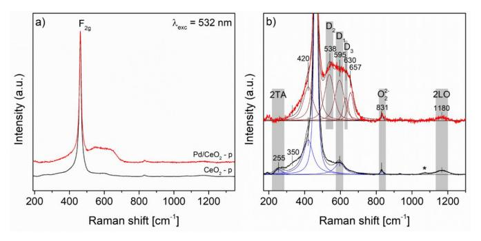
**Figure 3.** (a) General and (b) detailed views of Raman spectra of ceria polycrystals before and after palladium impregnation. All spectra have been normalized to the  $F_{2g}$  peak and vertically shifted for clarity.
