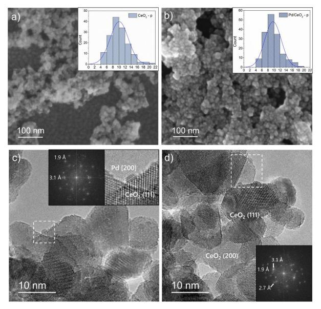
**Figure 1.** SEM images of ceria polycrystals (**a**) before and (**b**) after Pd deposition (Pd/CeO<sub>2</sub>), and (**c**,**d**) HRTEM images of the Pd/CeO<sub>2</sub> catalyst with their corresponding Fourier transform (FT) images.
