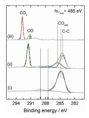
**Figure 7.** *Operando* XPS spectra of C 1s recorded over Pd/CeO<sub>2</sub> catalyst during CO oxidation under the following conditions: (i) reduction under 1 mbar of H<sub>2</sub> at 350 °C, (ii) 1 mbar pressure of CO at 250 °C, and (iii) CO oxidation under 1.5 mbar total pressure of CO:O<sub>2</sub> = 2:1 at 250 °C.
