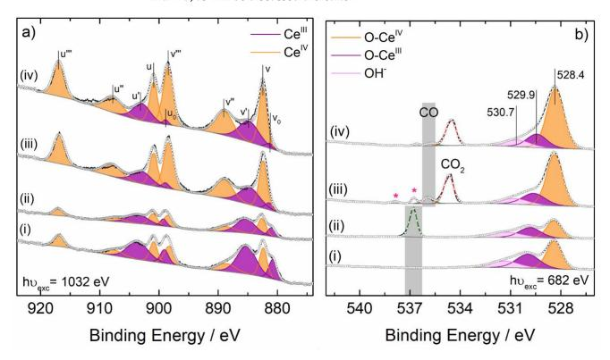
**Figure 5.** (a) *Operando* XPS spectra of Ce 3d and (b) O 1s recorded over Pd/CeO<sub>2</sub> catalyst under the following conditions: (i) reduction under 1 mbar of H<sub>2</sub> at 350 °C, (ii) 1 mbar pressure of CO at 250 °C, (iii) CO oxidation under 1.5 mbar total pressure of CO:O<sub>2</sub> = 2:1 at 250 °C, and (iv) CO oxidation under 1.5 mbar total pressure of CO:O<sub>2</sub> = 2:1 at 250 °C, and (iv) CO oxidation under 1.5 mbar total pressure of CO.
