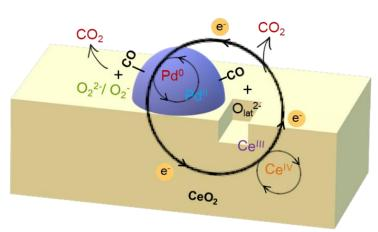
**Figure 10.** Illustrative scheme of the suggested electron transfer model for the CO oxidation reaction occurring on the Pd/CeO<sub>2</sub> surface catalyst.
