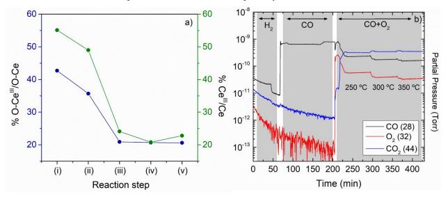
**Figure 6.** (a) Amount of reduced ceria measured at each reaction step from O 1s spectra at 682 eV (left axis) and Ce 3d spectra at 1032 eV (right axis) of the Pd/CeO<sub>2</sub> catalyst and (b) corresponding partial pressures of  $O_2$ , CO and CO<sub>2</sub> monitored by mass spectroscopy.
