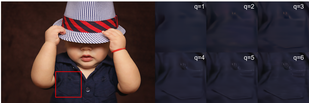
Figure 23: Left: Original RGB image with a red rectangle in the region to be cropped. Right: Reconstructed regions for the quality factor indicated in each subimage.
