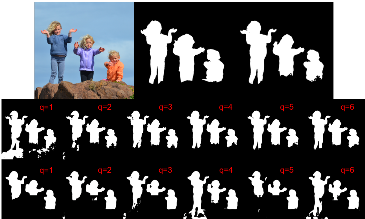
Figure 51: First row: RGB image, ground-truth and original anchor prediction. Second row: decoded anchor prediction for each quality level. Third row: latent code approach prediction for each quality model.
