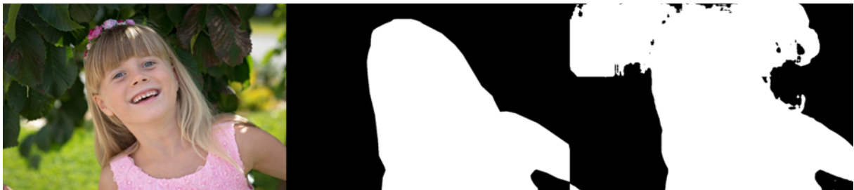
Figure 17: Left: RGB image. Center: Ground truth. Right: Predicted mask with an accuracy of 0.7697 and mIoU of 0.6208.
