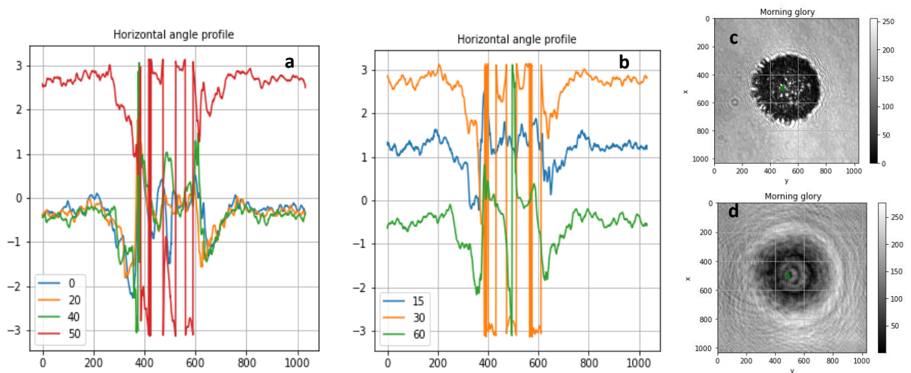
Fig.19: (a) & (b) In these images we see the angle information on the y axis and the space that goes through the middle (dot green in (c)). The different lines correspond to different propagation distances. (c) Raw Morning glory hologram used for obtaining the information (d) Propagated morning glory hologram.
