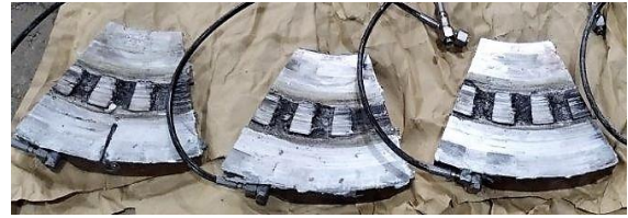
Fig. 3. Bearing pads with damage
