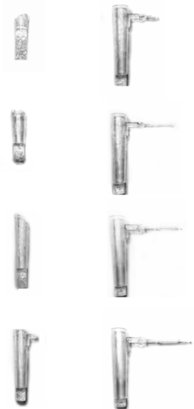
Figure 3.14: Filling study of a COP polymer with nodal point. Short shots at different filling times (from upper left to lower right)
