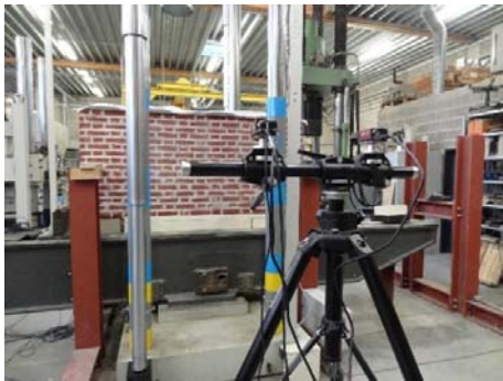
Figure 3: setup of two camera's for DIC measurements
