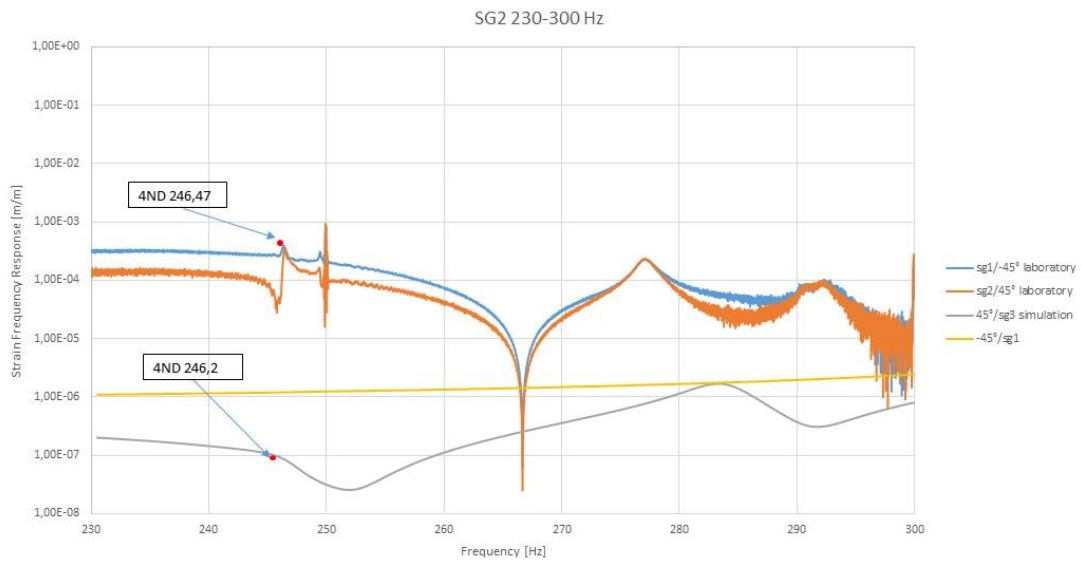
Figure 60 Strain gauges signal from laboratory and simulation for SG2
