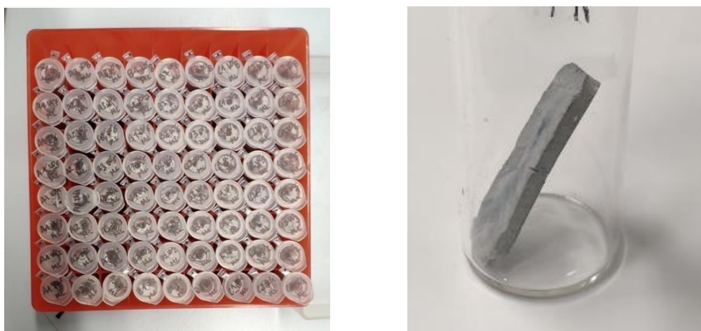
Figure 19. Sample preparation and storage for the swelling and degradation tests (left) and a hydrogel A (PEDOT:PSS + TA) dry sample after lyophilization
