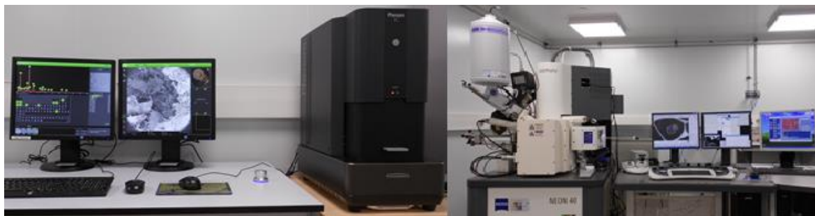
Figure 11 PhenomXL Desktop SEM (left) and Neon40 Crossbeam (right) used to perform visual examination of the samples
