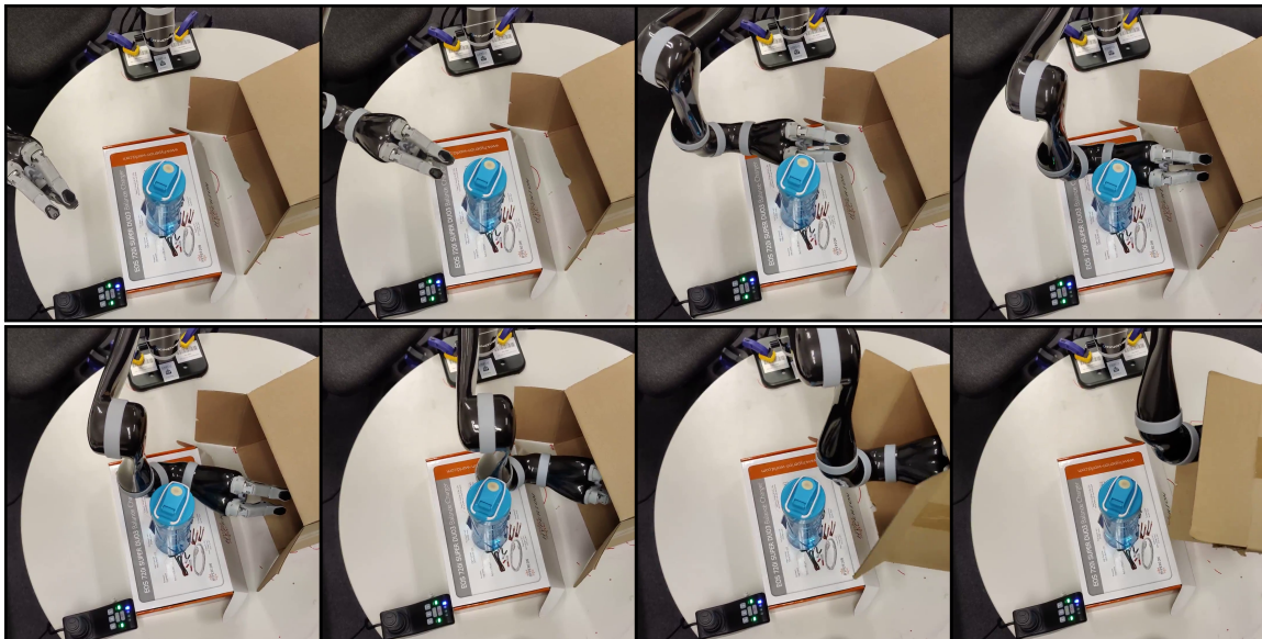
Figure 8.1: A motivating application for our work is generalising stable systems learned from expert demonstrations, when surroundings change. Here, a 6 degrees-of-freedom JACO arm is shown 8 recorded human demonstrations. Then, an obstacle bottle is placed right in the path of the recorded demonstrations. The JACO arm is able to warp smoothly around obstacle and successfully reach in and lift the box.
