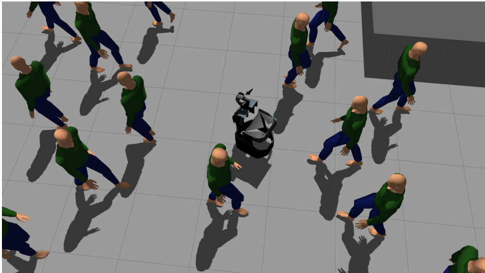
Figure 5.1: A non-holonomic robot drives towards a goal while interacting with pedestrians and static obstacles, and actively adapts to probabilistic predictions of surrounding movements.
