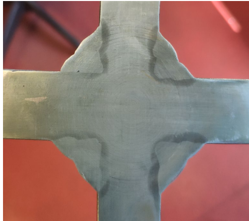
Fig. 2. Photo of the macroetched surface of a F12 specimen.
