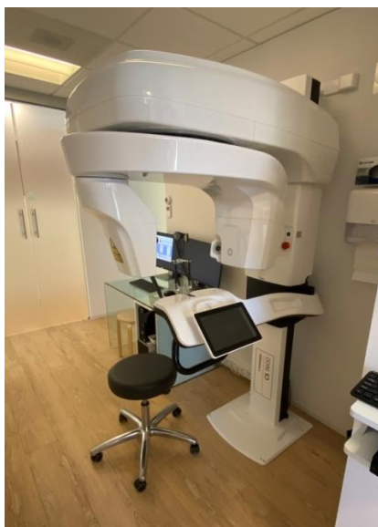
Figure 1.3: dental cone beam computed tomography machine.
