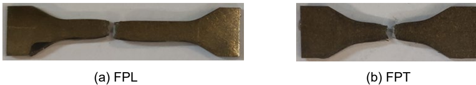
Fig. 9. Fractured miniature flat plates for base metal.
