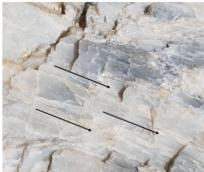
Figure 5. Longitudinal and elongated tabular cleavages can be seen in this photograph of a high grade spodumene ore sample from Bald Hill mine site in Western Australia (Tadesse et al., 2019)
