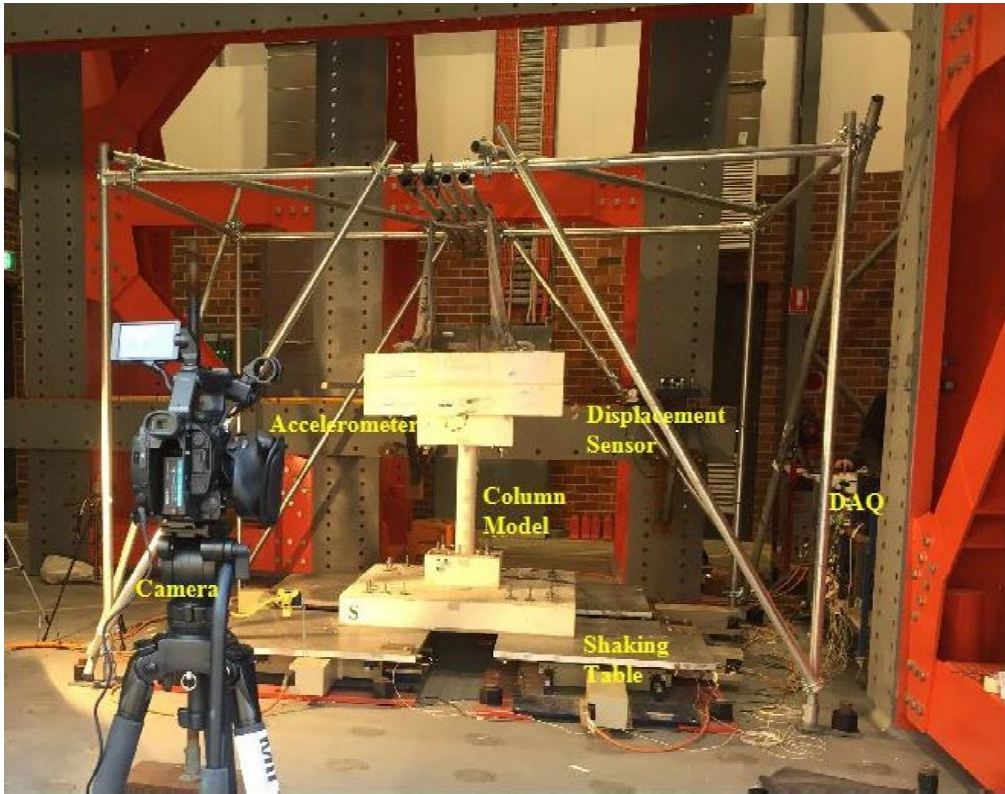
Figure 4: Experiment setup for the proposed vision-based vibration measurement.
