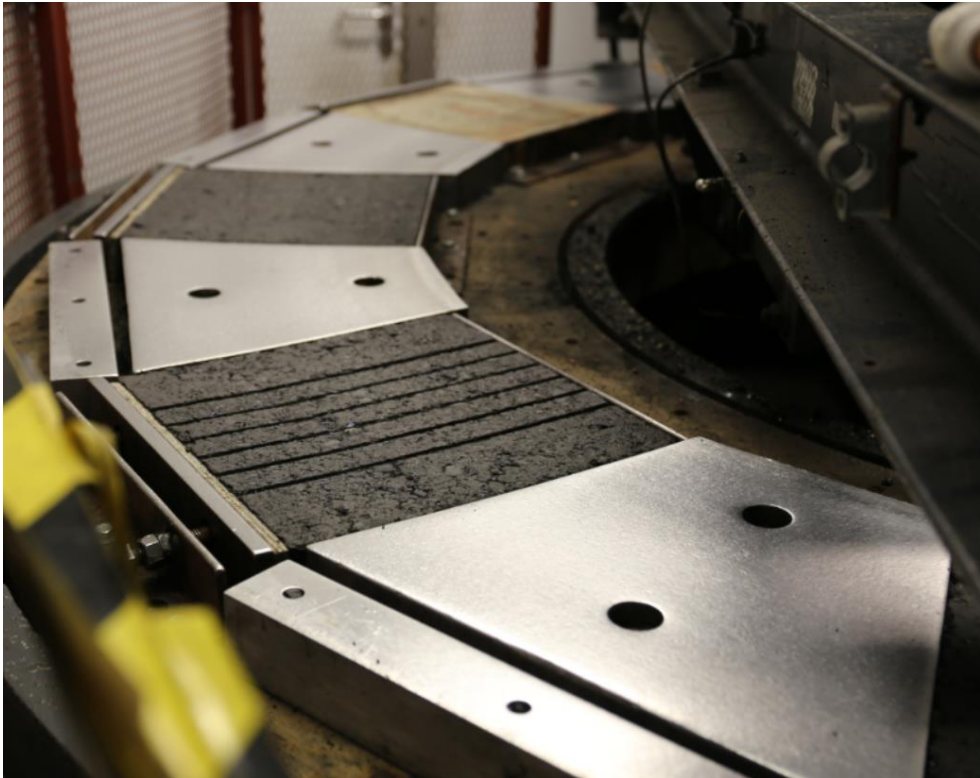
Figure 3.2. Grooved Marshall Asphalt Test Specimen in the RTM.
