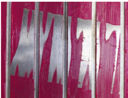
Figure 9.10. Contact phenomena for the pendulum on 38mm ribs and 6mm groove pattern at 9°
