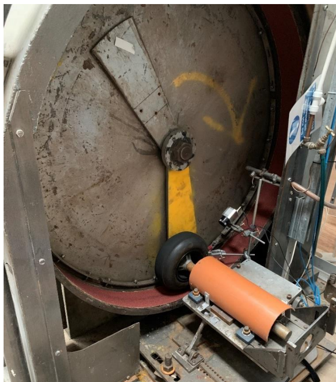
Figure 3.7. The Ulster Loaded Tyre Road Assimilator.
