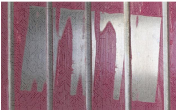
Figure 9.9. Contact phenomena for the pendulum on 38mm ribs and 6mm groove pattern at 6°
