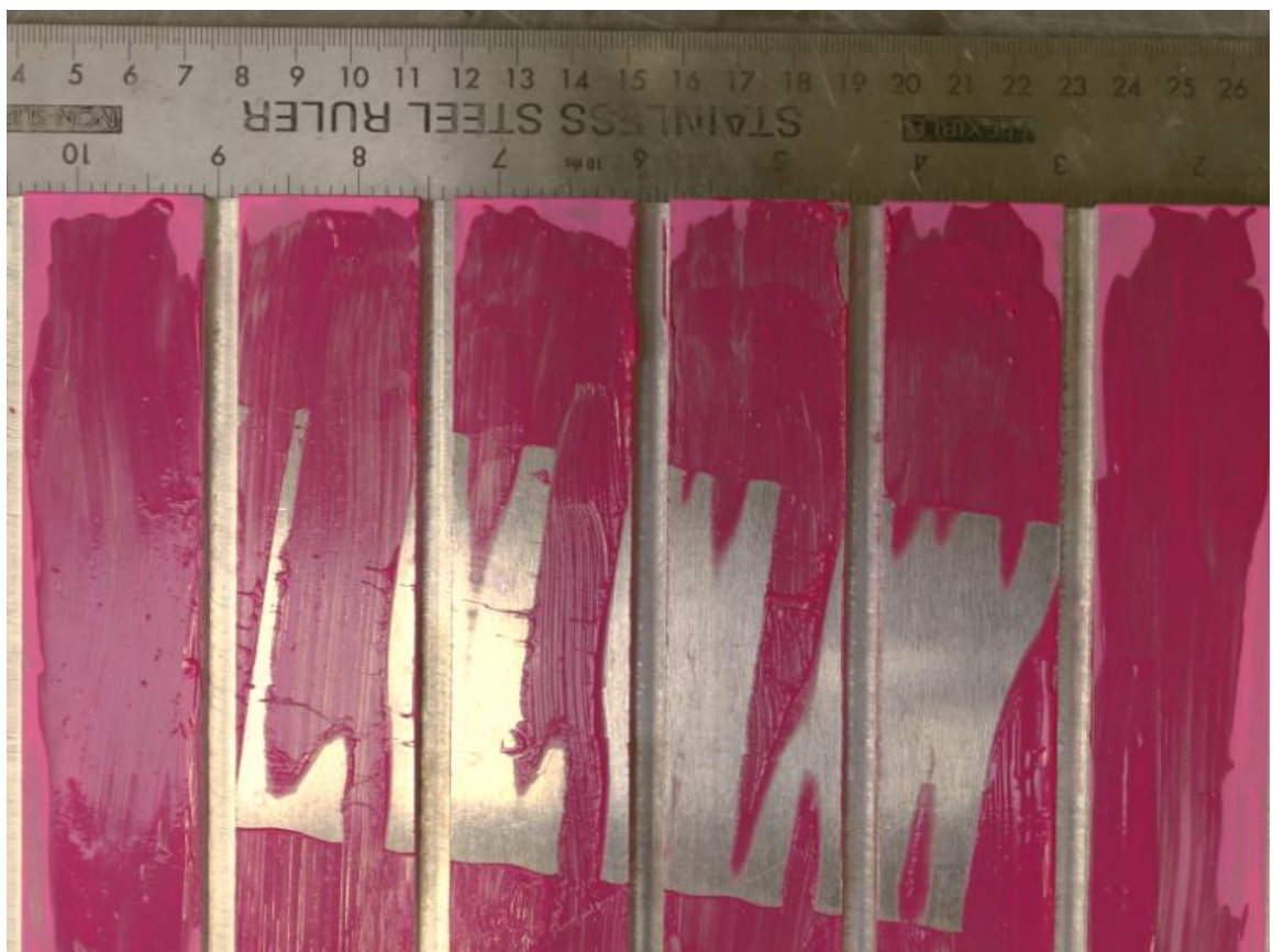
Figure 9.4. Paint removal for 6 mm groove width and 32mm rib width at 10°.
