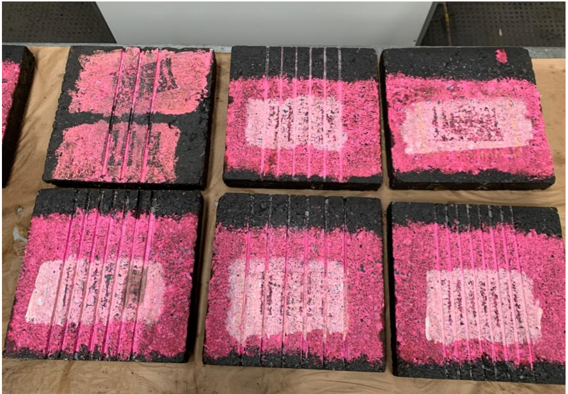
Figure 4.7. A selection of the grooved MA test surfaces
