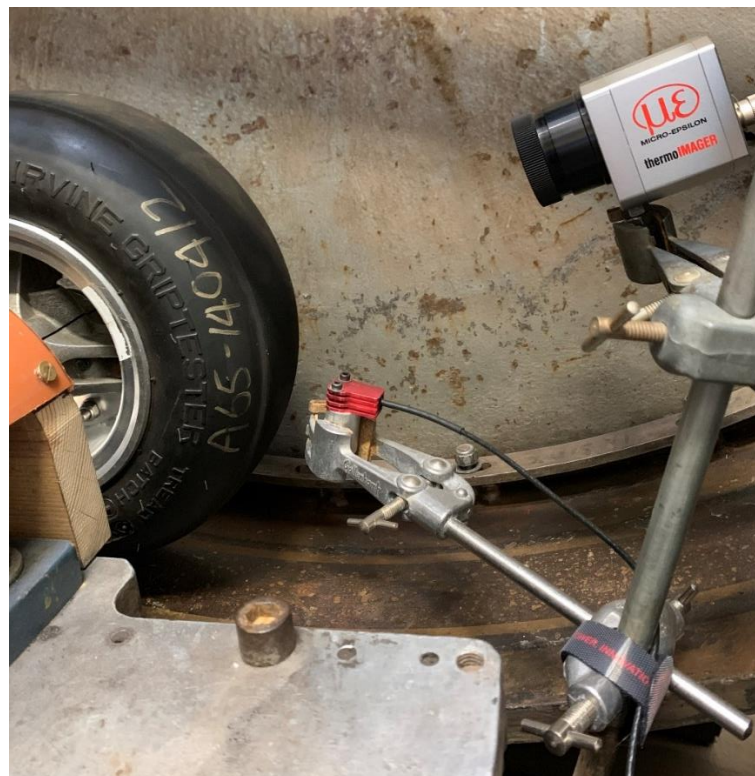
Figure 10.3. Impact temperature measurement set up
