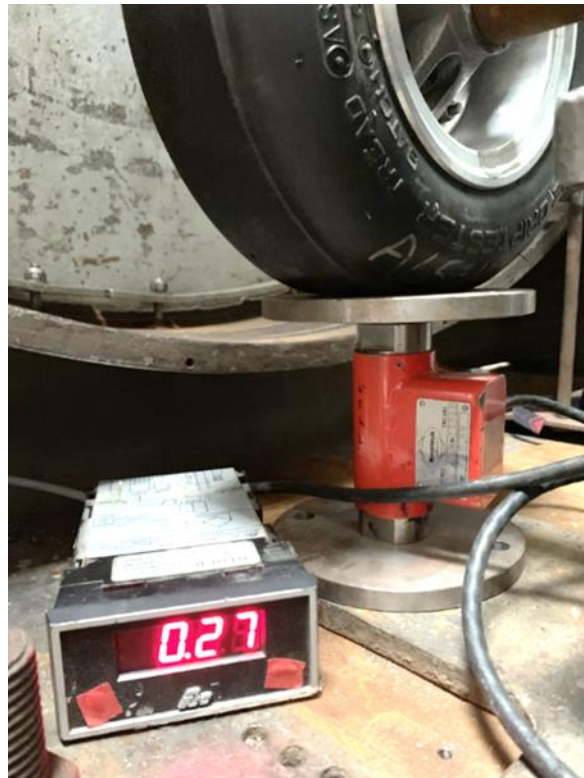
Figure 10.2. Determination of total static vertical load using Novatech F204 load cell with a digital Red Lion strain gauge indicator
