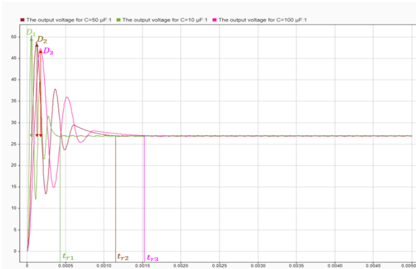
Fig. 5. Evolution of the output voltage of the converter according to the variable capacitance C.
