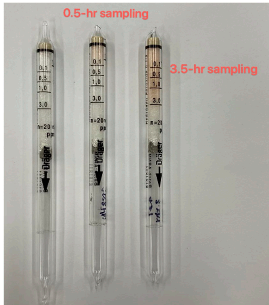
Figure 5. Results from colorimetric sampling with a H 2 O 2 Dräger-Tube installed downstream of the air cleaner: before sampling, after 0.5 h, and after 3.5 h of sampling.
