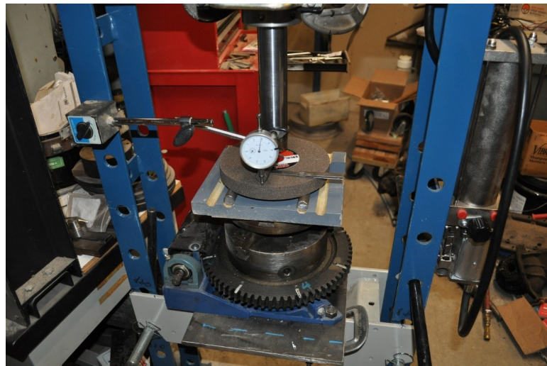
Figure 2. Three-point bending fixture to crack the grinding wheels.
