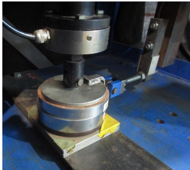
Figure 5-2: Modified Jenike shear tester arrangement
