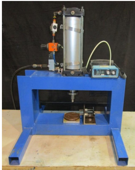
Figure 5-1: Consolidation Station used to apply twisting to sample
