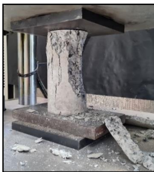
Figure 4: Comp. Test - Normal Concrete
