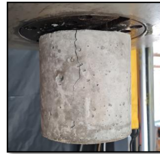
Figure 9: Anchor Pullout Test Test Machine
