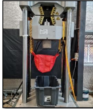
Figure 8: Anchor Pullout Test – Universal Load
