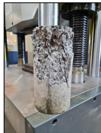
Figure 11: RPA Remained Intact Post Failure due to Compression
