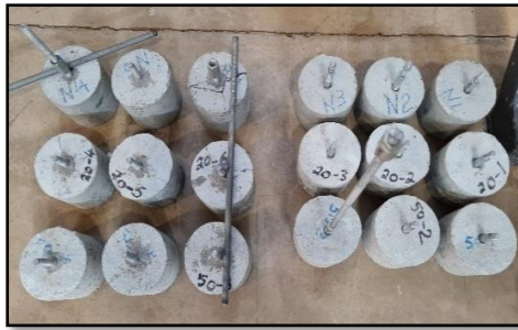
Figure 7: Samples (Mech. & Chem. Anchors)
