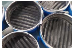
Figure 6: Greased artificial rock joint moulds
