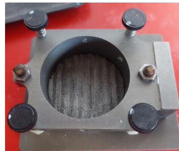
Figure 8: ShearTrac2 Shear Apparatus Figure 9: Alignment of bottom joint in shear box
