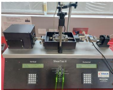
Figure 8: ShearTrac2 Shear Apparatus Figure 9: Alignment of bottom joint in shear box
