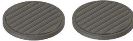
Figure 5: 3D model of interlocking sawtooth mould
