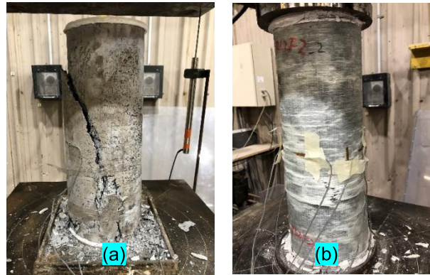
Figure 3: Failure modes of plain and FRP confined columns
