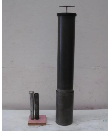
Figure 10: Drop hammer equipment used in coal toughness testing
