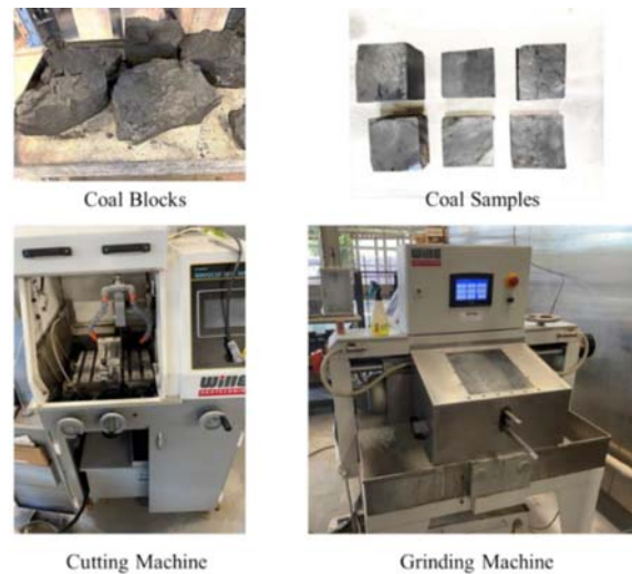
Figure 3: Coal samples prepared via cutting and grinding
