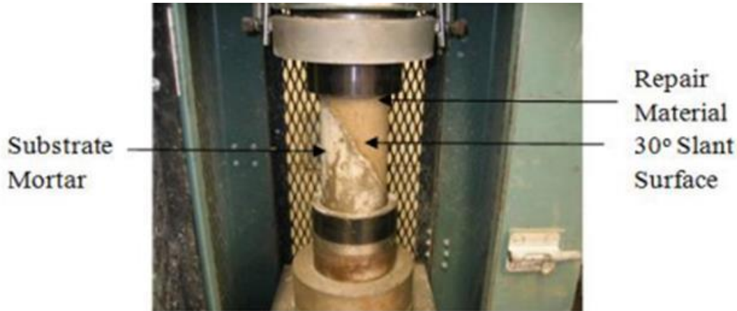
Figure 3: ASTM C882 Slant Shear Test methodology (from Yates pers com 2022)
