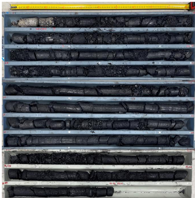
Figure 11: Core recovered from the angled hole pre-injection
