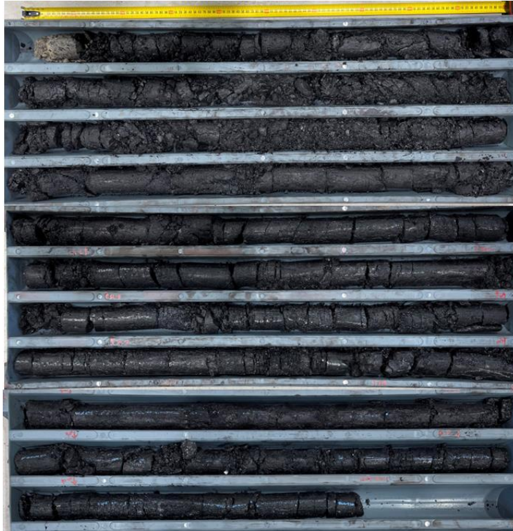
Figure 10: Core recovered from the horizontal hole pre-injection
