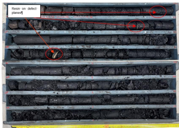
Figure 13: Core recovered from the angled hole post injection
