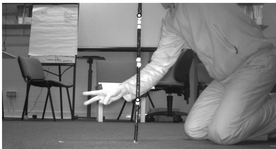
Figure 6. A camera calibration image with pole in position 2 m from the camera.
