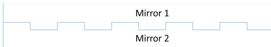
Figure 4. Layout of staggered mirrors creating a slit mirror array.
