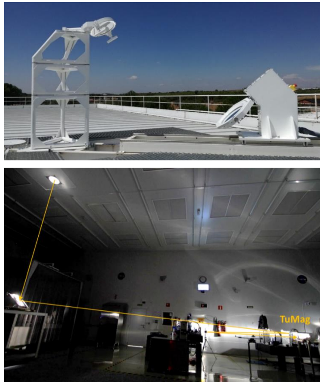
Figure 3. Up) INTA coelostat. The stabilized Sun light is directed towards the clean room. Bottom) Folding mirrors and imaging system in ISO6 clean room.
