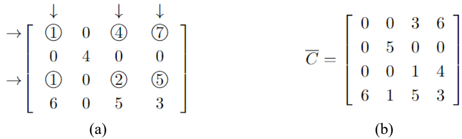
Figure 4. Illustrating the dual variable update: (a) Using \bar{C} for finding \delta and updating the dual variables. Arrows indicate that i \in SU and j \in V \setminus LV resulting in a \delta = 1 ; (b) updated \bar{C} using the new dual variables u = (5 \ 6 \ 5 \ 3) and v = (4 \ -1 \ 1 \ 0) .
