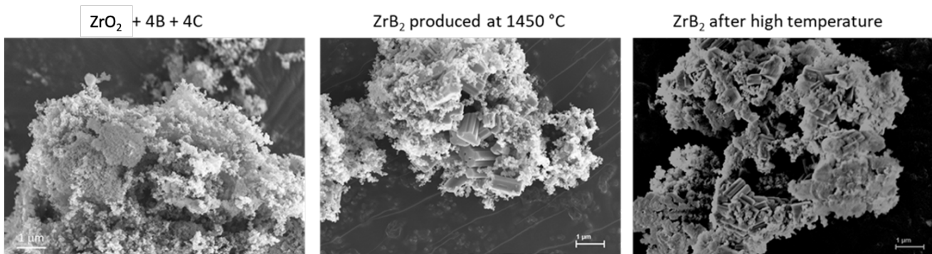
Figure 9. Mixture of precursors denominated 1:4:4 (left), after fabrication of ZrB_2 (middle) and after torch treatment (right).
