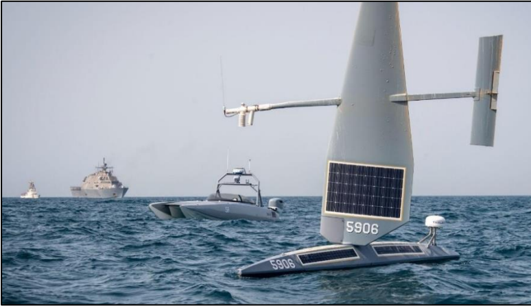
UxS Saildrone Explorer using solar technology as its energy source.
