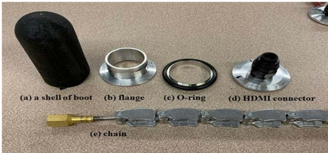
Figure 8. Components used for assembling sensor housing
