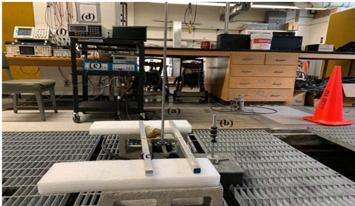
Rod (a), speaker (b), rotator (c), rotator controller (d), MFLI lock-in amplifier (e), and power amplifier (f).
