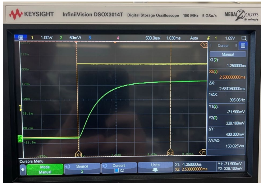
Figure 33. Single Pulse Transient Response of Prototype Circuit
