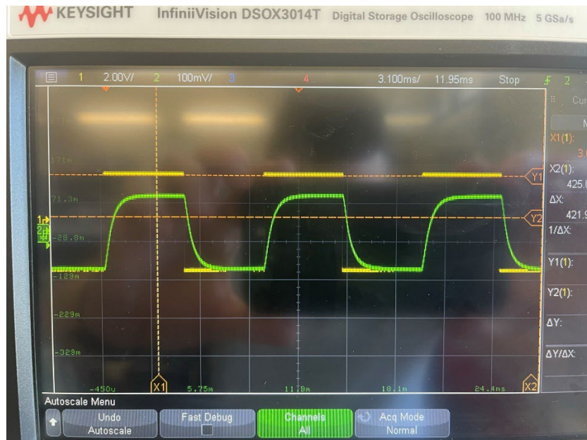
Figure 34. Multi Pulse Transient Response of Prototype Circuit
