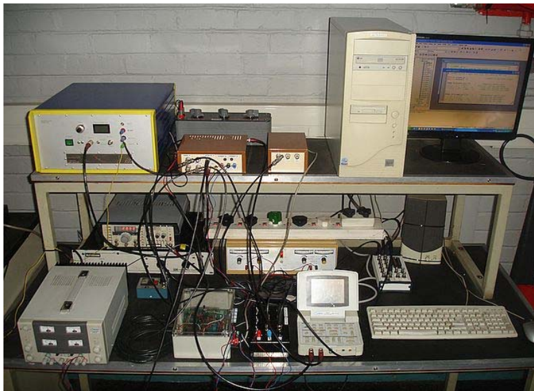
Figure H.2.: Instrumentation bench: Lower surface front left to right: \pm 15 V Dual power supply, DSP, 8 kHz anti-alias filter, digital oscilloscope. Lower surface middle: Piezotronics power unit (blue). Lower surface back left to right: Function generator (top left) shaker drive amplifier (bottom left), \pm 25 V dual power supply, connector block. Top surface left to right: Piezo drive amplifier, sensing circuit (front), adjustable polystyrene capacitor (back), reference capacitors.
