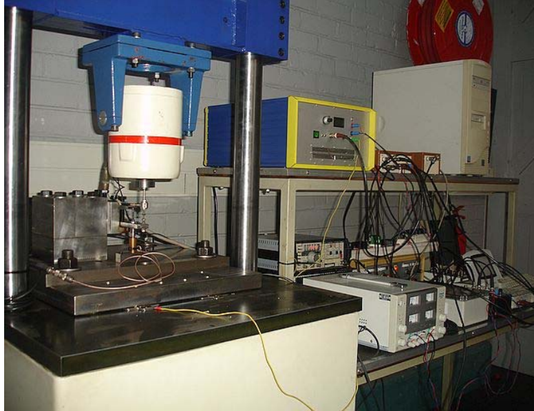
Figure H.1: Set-up: Shaker with self-sensing actuator (copper casing) and representative tool post and holder left and instrumentation bench right.
