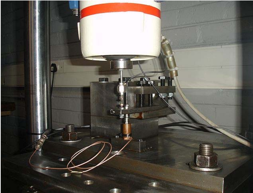
Figure H.3: Connection of shaker via load cell and stinger to representative tool holder supported by self-sensing actuator and clamped in representative tool post
