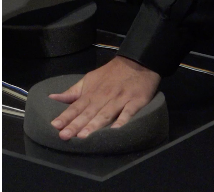
Figure 22. Low-density foam covering a force-sensing resistor
