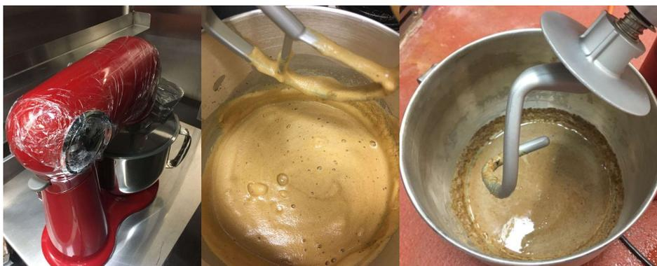
Figure 51. Photographs of various scale-up tests in the stand mixer: stand mixer placed in the blast chiller (left), 1 L of “whipped” BSG solution (center), 1 L of BSG solution (right).
