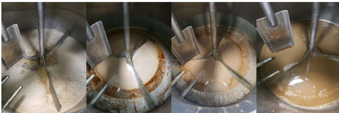
Figure 50. Photographs of various scale-up tests in the stainless-steel reservoir: lot 1, 100 L (left); lot 2, 25 L (center left); lot 3, 25 L (center right); lot 4, 50 L (right).
