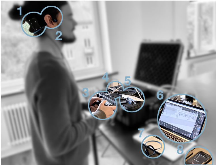
Fig. 5.2: Virtual reality system, Parrot-VR, test setup: 1) inertial measurement unit; 2) bone-conductive headphones; 3) controller; and 4) embedded computer. Auxiliary equipment: 5) audio interface; 6) laptop; 7) bone-conductive headphones; and 8) audio recording device. Figure and caption reprinted from [163].
