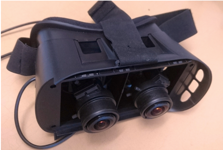
Fig. 7.4: Attempted, and later abandoned, prototype for a sensor solution utilizing stereo-vision in 2017.
