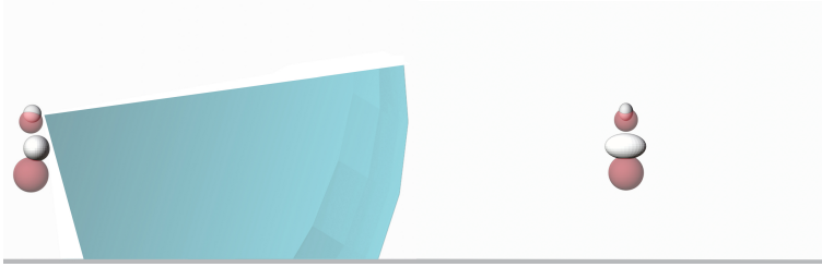
Fig. 5.3: Virtual reality avatar in default positioning, from the side and front. White spheres are head and body, and red their pivot points, blue cone is the sensor field-of-view (not visible on the right). The body can affect the sound feedback by occluding this, which happens for many possible head rotations. All sizes and relative positions that might affect this are based on a hypothetical female user with relevant features at the most disadvantageous 95th percentile of anthropometric data. Figure and caption reprinted from [163].
