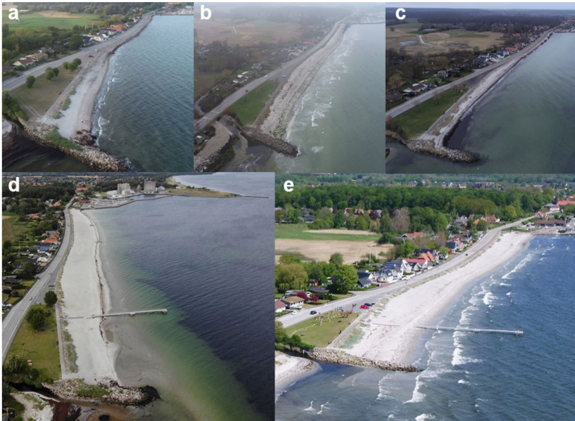
Figure 3: Drone images of Faxe Ladeplads towards the NE. The nourished area is the stretch between the harbor and the terminal groin. (a) August 2018, before the initial nourishment, (b) December 2018, just after the initial nourishment, (c) March 2020, (d) July 2021, just after the re-nourishment, (e) May 2022, including down-drift area. (Images: (a-d) Danish Coastal Authority, (e) Authors.)
