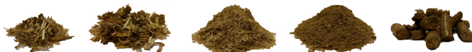
Figure 6 Mechanically pretreated straw. From left to right: chopped, roll milled, hammer milled, extruded, and pelletized.
